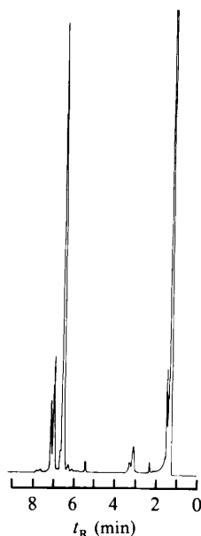
Fig. 1. Capillary GLC of the acetylated sterol fraction of N. exedens . The peaks of the three sterol acetates are between t_R 6.5 and 7.5. A sychromat with a quartz capillary (25 m \times 0.35 mm) containing OV-1701 was used.
