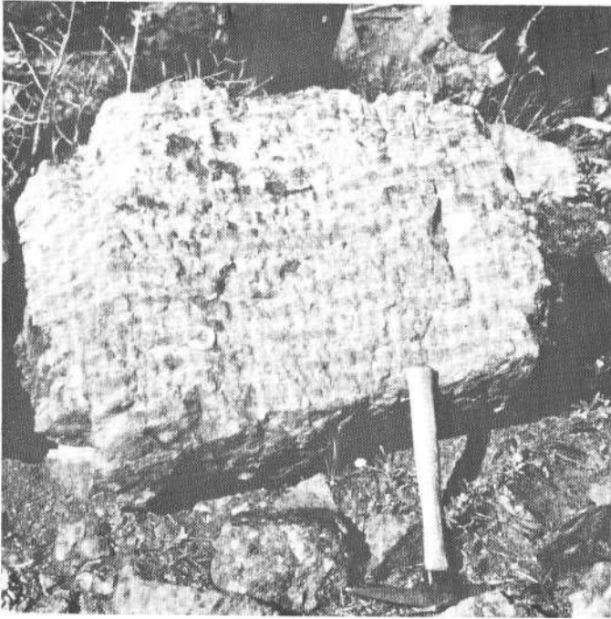
FIGURE 46.—Olivine cumulate with flattened bronzite oikocrysts.
