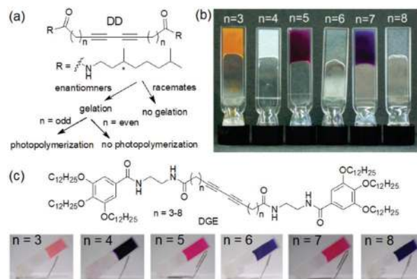
Fig. 15 (a) Illustration of gelation ability of diacetylene diastereomers (DD). 179 (b) Photographs of the cyclohexane gels of diacetylene diastereomers (DD) after photoirradiation. Reprinted from ref. 179 with permission from the American Chemical Society, copyright 2004. (c) Structures of the diacetylene–gallic ester conjugate (DGE) gelators and photographs of DGE gels after photoirradiation. 180 Reproduced from ref. 180 with permission from the American Chemical Society, copyright 2007.
