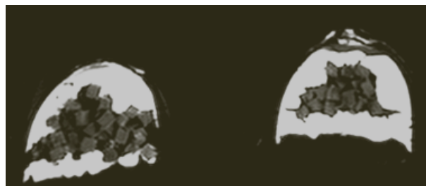
Figure 4. MR image of the breast phantom. We can see at the center the turkey breast represented by the fibroglandular tissue and, in the periphery, the fat tissue represented by pork fat and jelly agents.
