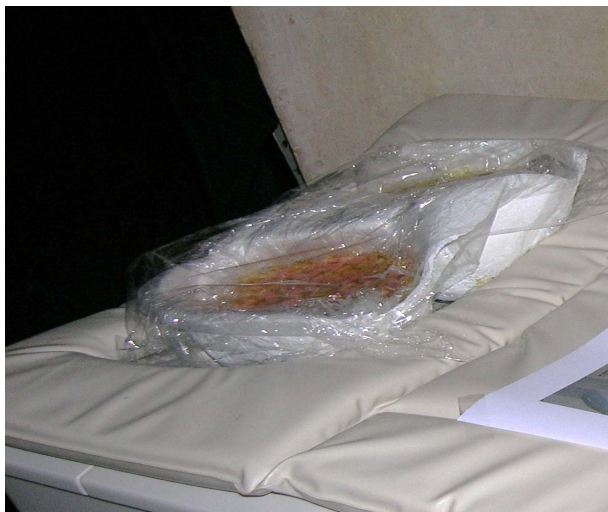
Figure 5. MRI breast phantom positioned inside the coil is a sensitive surface coil with a place to dovetail both breasts. The coil goes into the tunnel with the woman in ventral position. The prototype only differs on the weight and volume of the women trunk.
