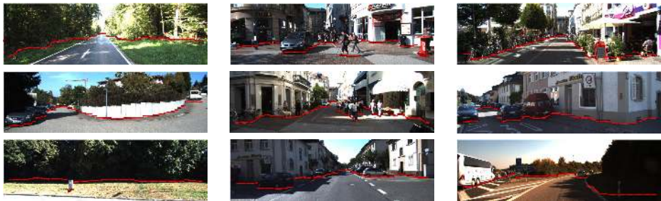
Figure 4: Obstacle detection results on test images (See section 4). the red dots mark the ground contact points of the general obstacles as computed using StixelNet and CRF.
