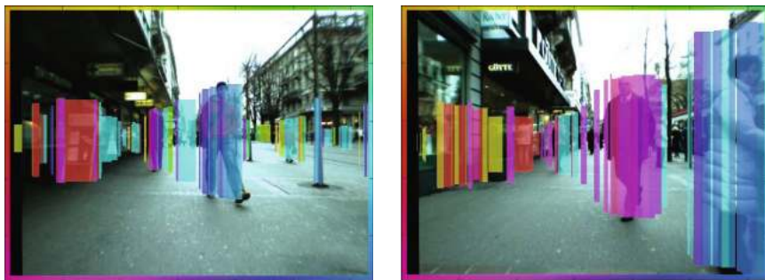
Fig. 6. Example results of our stixel motion estimation algorithm. Motion vector orientation is colour coded (see image border). Left image shows frame 8.
