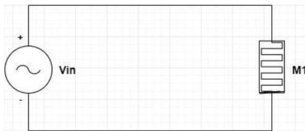
Fig. 4 Circuit used as a test setup to carry out SPICE simulations of all kinds of memristor models discussed in this paper
