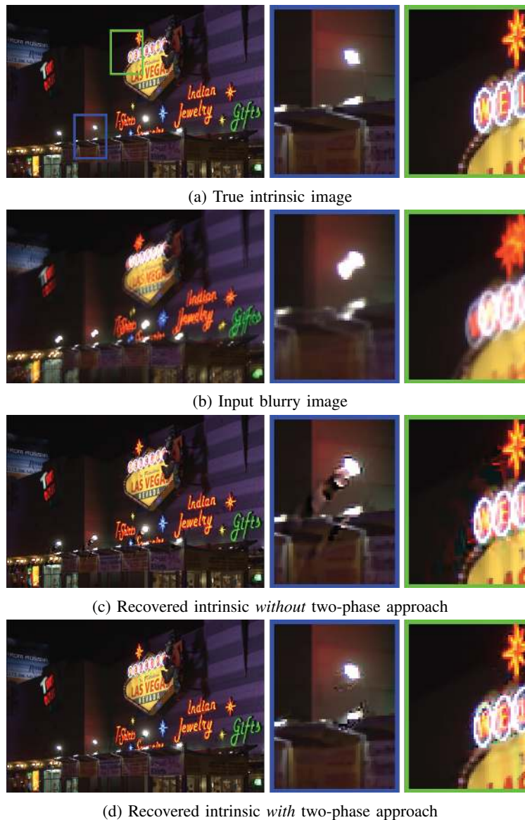
Fig. 12: Results on partially saturated image. The dynamic range of pixel intensities in the true intrinsic image is [0, 68] . The simulated blurry image is clamped to 1. The proposed two-phase approach helps reduce ringing artifacts near saturated pixels.
