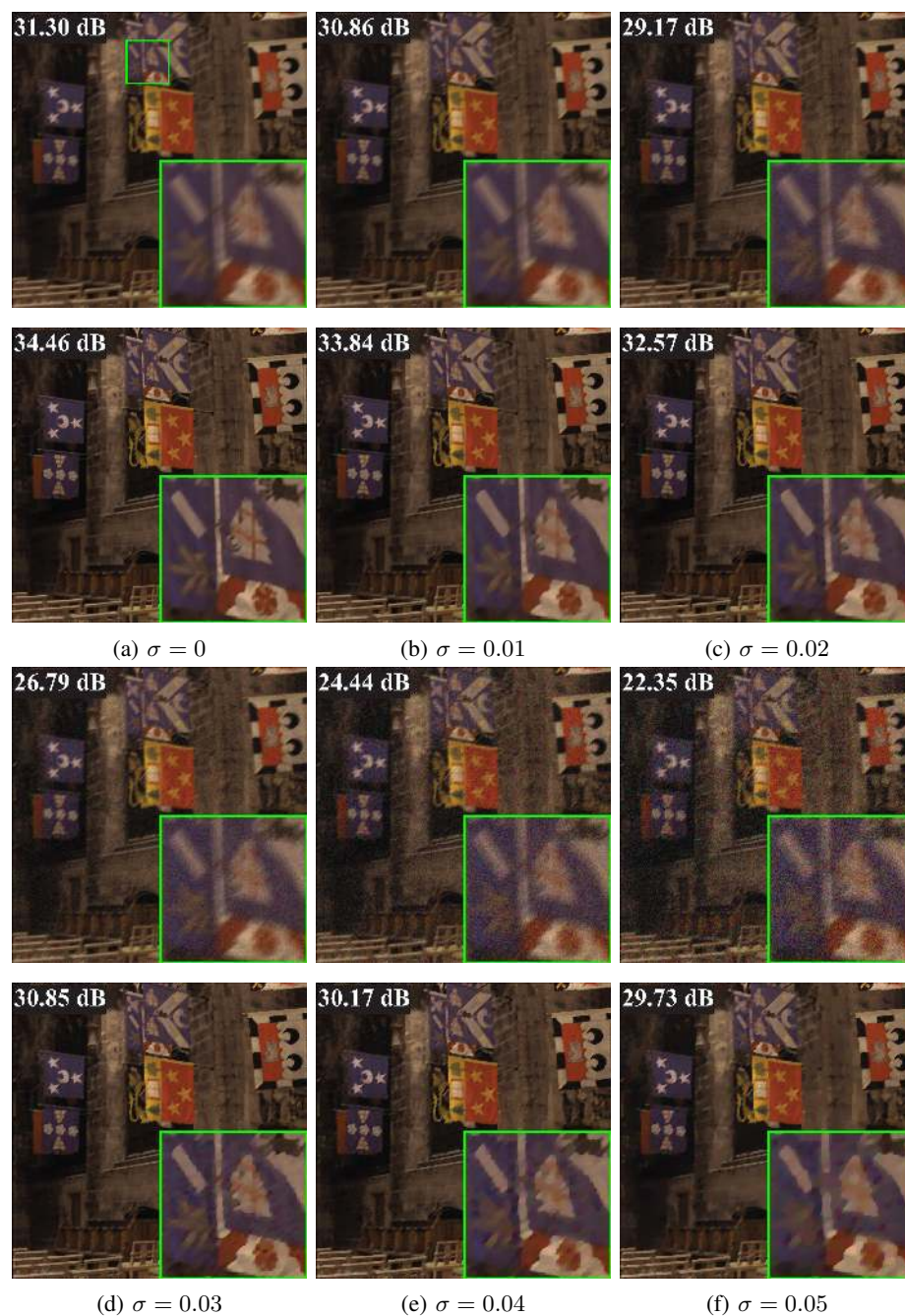
Fig. 15: Results on synthetic data with difference levels of white Gaussian noise. In subfigure (a-f), the standard derivation ( \sigma ) of the noise is set to be 0, 0.01, 0.02, 0.03, 0.04 and 0.05 respectively. In each subfigure, the 1 st row shows the input blurry image, and the 2 nd row shows our deblurred result. The PSNR values are shown at the left-top corner of each image. An inset is shown at the right-bottom corner of each image for better view.
