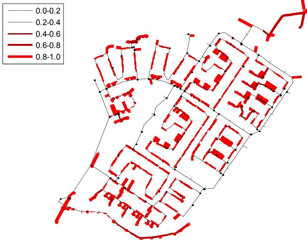
Figure 8-5. Percentage of time that pipe flow is stagnant pipes (0.01 h time step).
