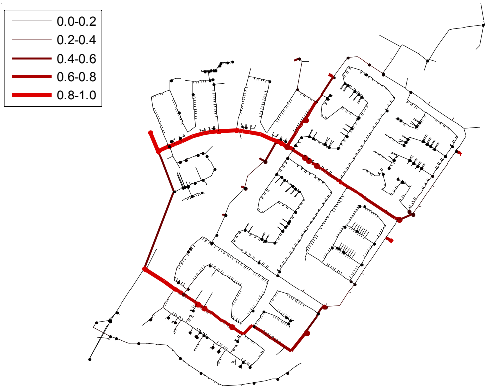
Figure 8-7. Percentage of time that pipe flow is turbulent pipes (0.01 h time step).
