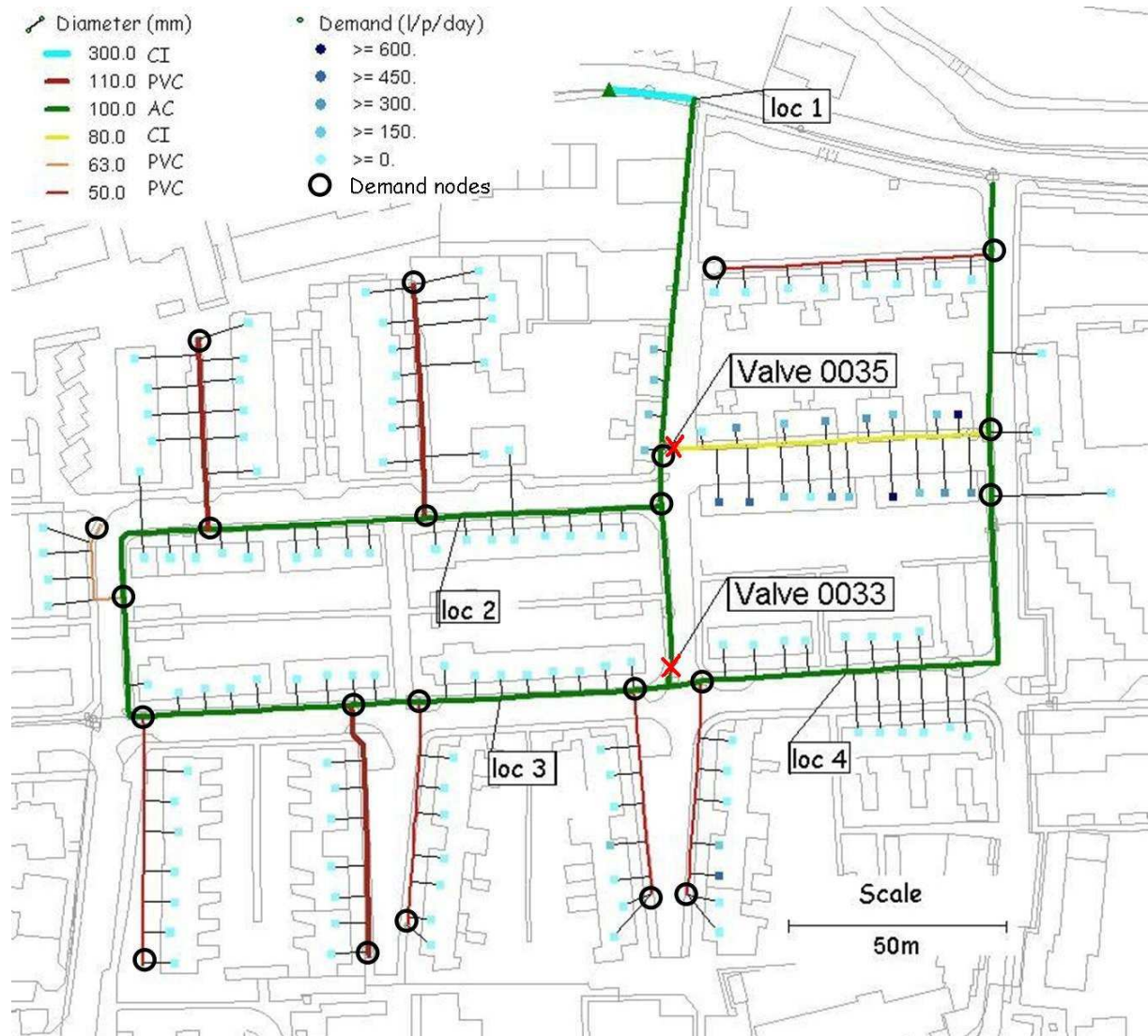
Figure 6-1. Network layout. Water enters at location 1. Valves 0033 and 0035 are closed in the branched layout and open in the looped layout. Valve 0035 is placed at the 80 mm CI main.
