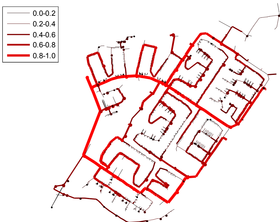
Figure 8-4. Cross-correlation of incoming flow and flow in all pipes (0.01 h time step).
