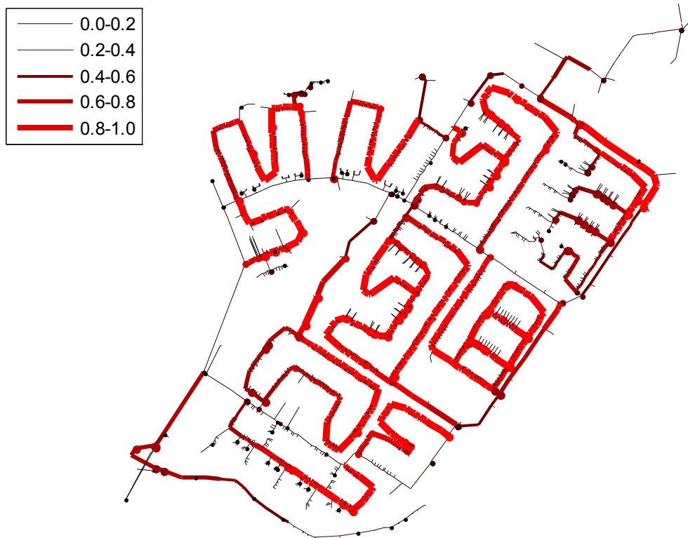
Figure 8-6. Percentage of time that pipe flow is laminar pipes (0.01 h time step).
