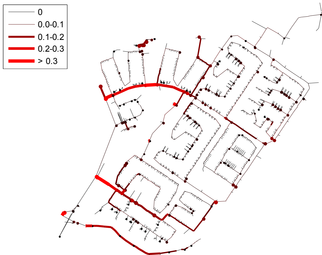
Figure 8-10. Maximum flow velocity (m/s) per main pipe; connection lines are not computed pipes (0.01 h time step).
