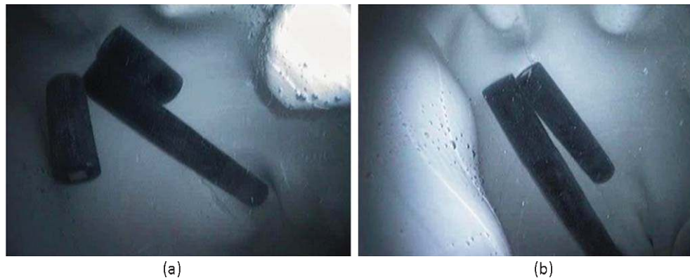
Fig. 11. Experiment No.3 showing assembled mock-ups in the stomach simulator: (a) before contraction (No-assembly: 2, three-assembled: 1) and (b) final configuration (Two-assembled: 1, Three-assembled: 1).
