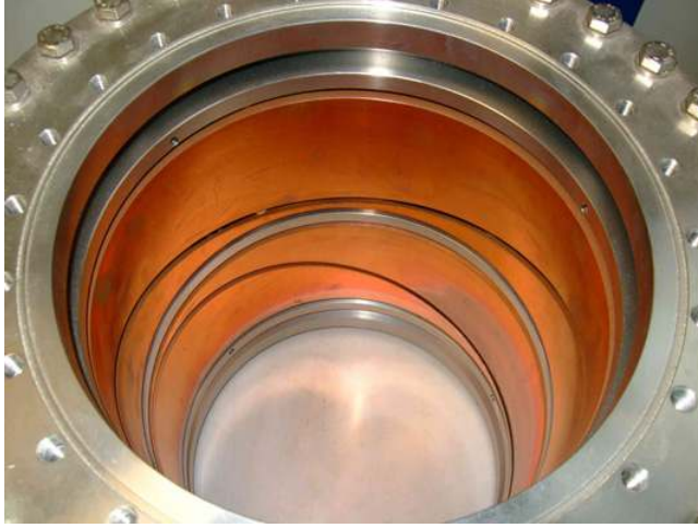
Fig. 70. Beam position monitor of the TSR.
