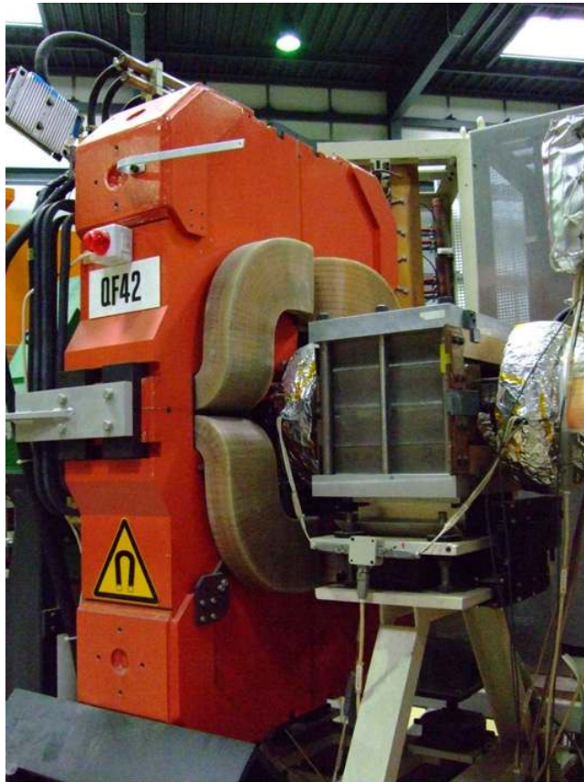
Fig. 31. TSR quadrupole magnet. In the front of the quadrupole magnet a bump magnet used for multi turn injection is visible.
