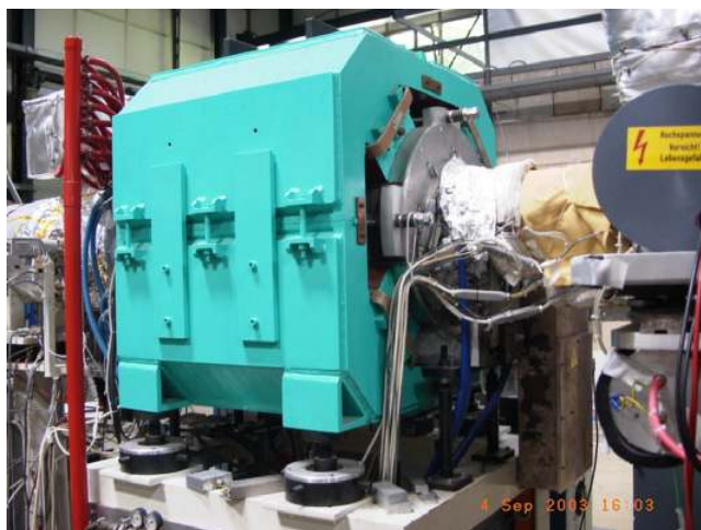
Fig. 54. The quadrupole ferrite loaded resonator.
