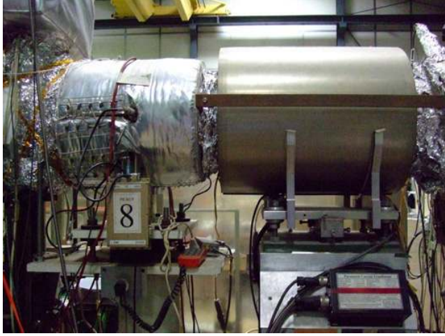
Fig. 77. Multilayer magnetic shielding of the current transformer housing the magnetic sensor (right). On the left side the thermal isolation of pick-up 8 is visible.
