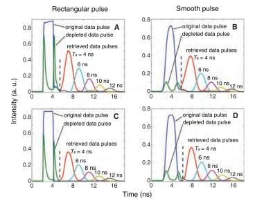
Fig. 3. Storage of pulse sequences. (A) shows experimental results for two 2-ns-long data pulses separated by 1 ns, and (C) shows the corresponding theoretical simulations. (B) shows the case of three 2-ns-long data pulses separated by 1 ns. with the corresponding simulations shown in (**D**). The retrieved pulses are shown with a multiplication factor of 5 to the right of the dashed vertical line. For clarity, the depleted data pulses are not shown.
