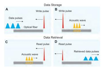
retrieval process (C), a short, intense read pulse at the same frequency as the write pulse depletes the acoustic wave and converts the data back to the original optical frequency, thereby producing a replica of the incident data pulses (D).
