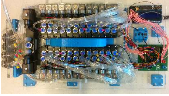
Fig. 6: Computer-controlled pneumatic distributor.
