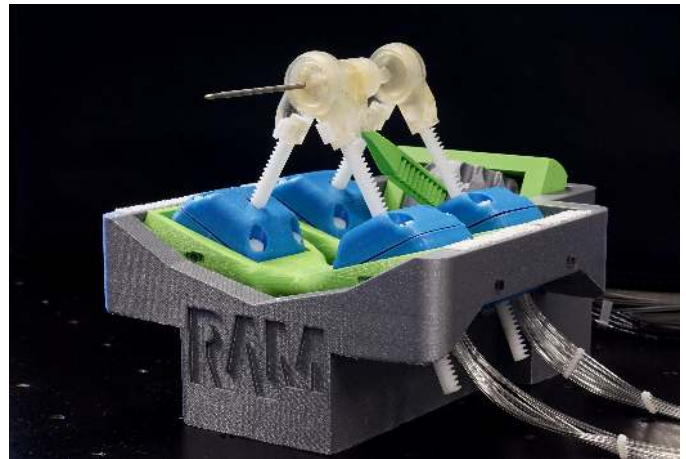
Fig. 1: The MRI-compatible biopsy robot Stormram 3.
