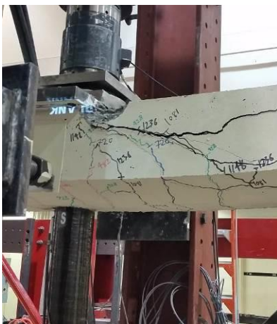
(a) Concrete crushing at top chord
