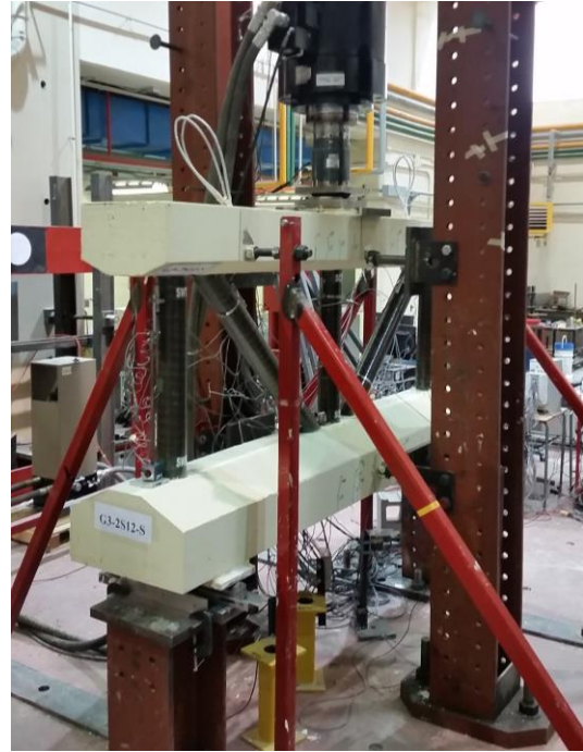
(b) Truss Girder during the Test
