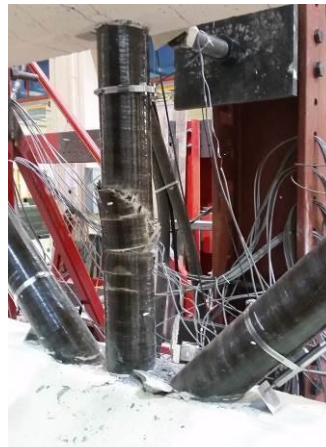
(b) Rupture of middle CFRT element
