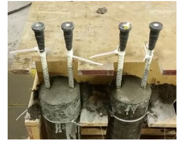
(c) Protruded Headed-Bars
