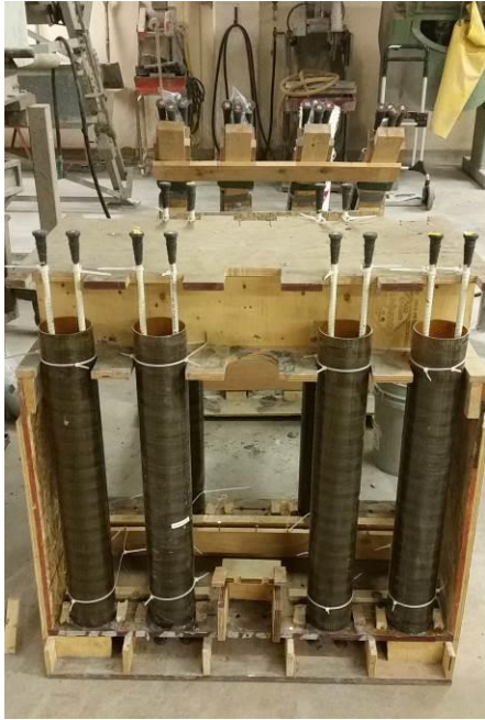
(a) Vertical Tubes before Casting
