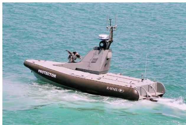
Figure 1: One example of an industrial-level USV is the remotely controlled Protector, developed by Rafael of Israel. This vehicle is a 9 m long rigid-hulled inflatable boat equipped with water jet propulsion that enables operations of up to 20 m/s (i.e., approximately 40 knots).
