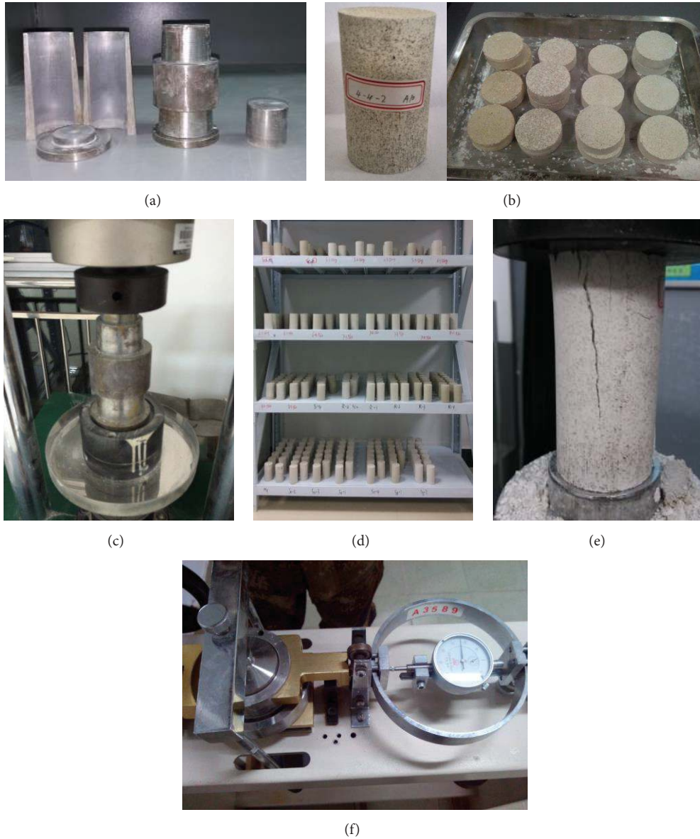
FIGURE 5: Equivalent materials and mechanical experiments: (a) the mould; (b) sample of equivalent materials; (c) sample preparation; (d) maintenance of the sample; (e) uniaxial compressive test of sample; (f) shearing test of the sample.
