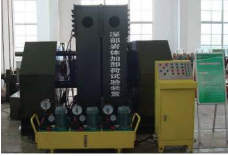
FIGURE 2: Deep rock mass loading and unloading test apparatus.
