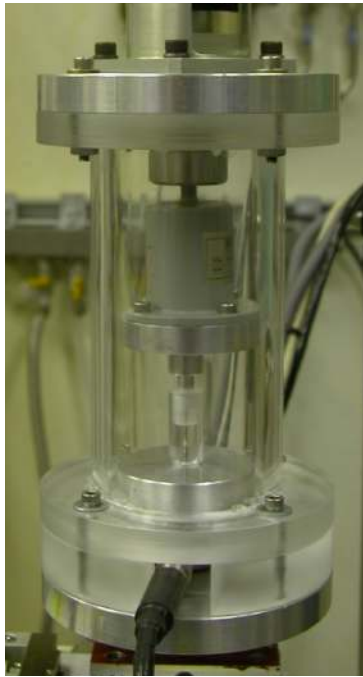
Figure 2. Photo and schematic of 1D compression test cell
