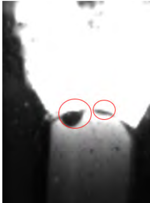
Fig. 5 Image of C-100 coated propellant. Red circles indicate melting of the coating.
