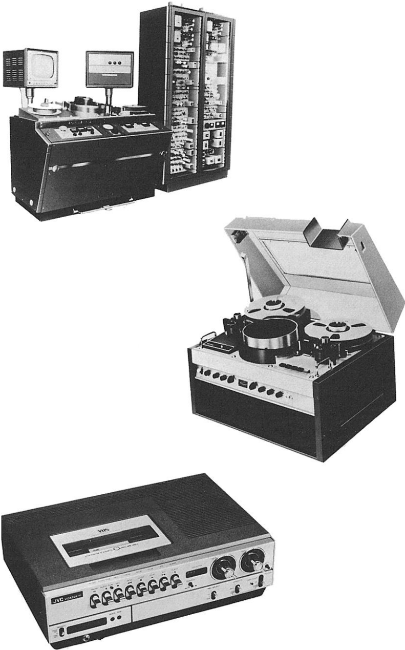
JVC Through the Years • The illustrations show the evolution of the VCR industry, from JVC's first helical recorder (top), through the bulky mid-1960s model often used by institutions, to the 1970s home VCR with which most consumers are familiar. (Photographs reproduced courtesy of JVC, Public Relations Department.)
