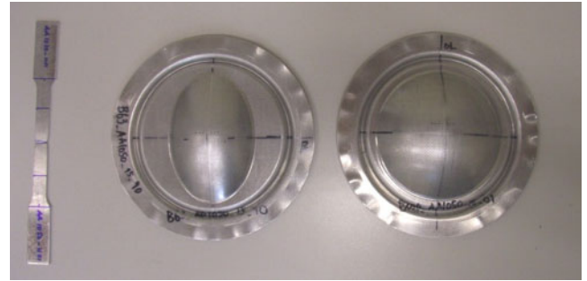
Fig. 2 Tensile, elliptical, and circular hydraulic bulge specimens utilized in the characterization of the formability limits of aluminium alloy AA1050-O
