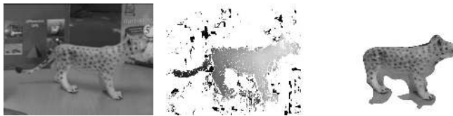
Fig. 6. Left) A left manipulation camera image, Middle) The corresponding disparity map, Right) Segmentation from mean shift in 3D space.
