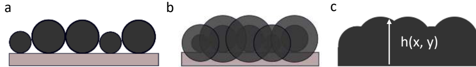
Fig. 3. Procedure to generate the rough surface template. Displayed is a two-dimensional cross-section of the three-dimensional height profile. a) Nanospheres are placed in a monolayer with the restriction that every nanosphere touches at least one other nanosphere. Overlapping nanospheres are not allowed. b) To mimic the isotropic coating by atomic layer deposition, the nanospheres are radially enlarged. c) The last step is to homogenize the resulting structure. The height profile is then the maximal height resulting from the enlarged nanospheres.
