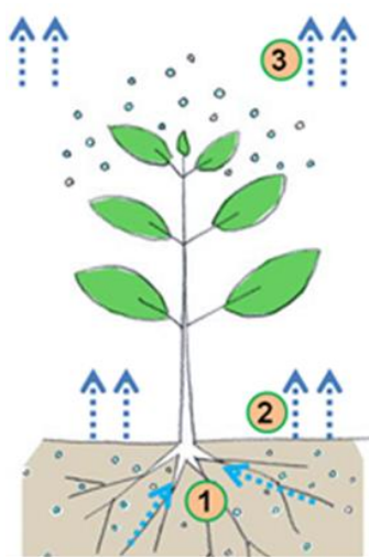
Fig.10. Schema of the humidification of the air by the urban tree, 1: Consumption of liquid water (Circulation of water), 2: Evaporation, 3: Evapotranspiration: corresponds to the evaporation of the water contained in the soil and transpiration from vegetation. (Latent heat flow) [11]
