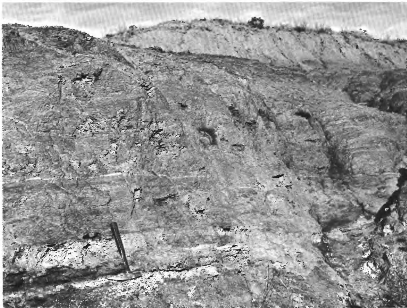
FIGURE 7. — Hard butters-weathering shale rich in organic material, fish scales, and bones in lower unit of Sharon Springs Member of Pierre Shale at locality 1. Hammer marks position of a 0.2-foot-thick yellowish-gray nonswelling bentonite bed.
