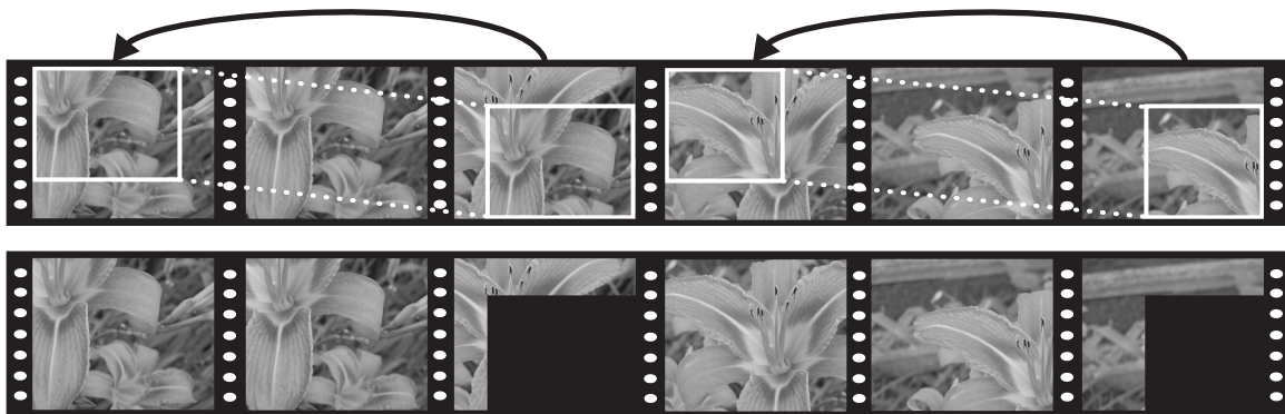
Figure 2-4: Eliminating temporal redundancy through forward motion estimation.
