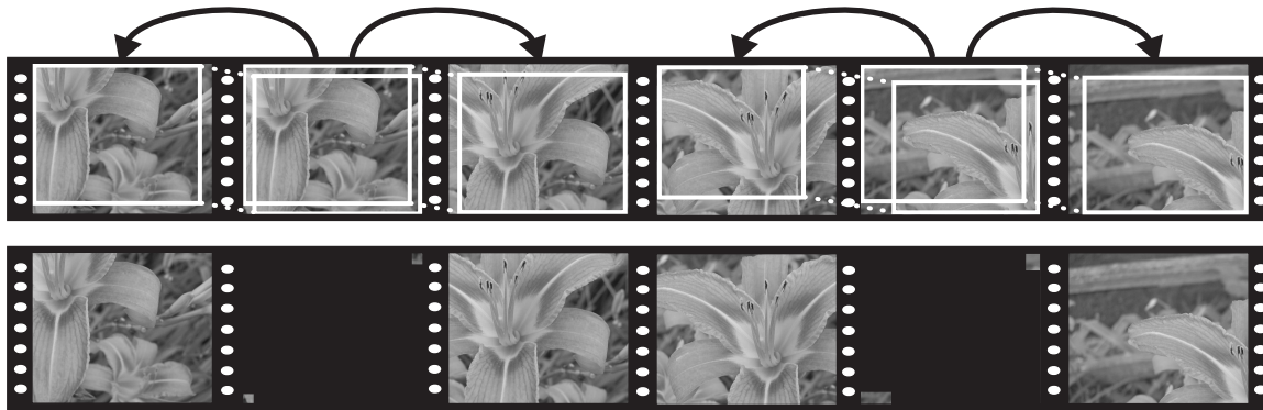
Figure 2-5: Eliminating temporal redundancy through backward motion estimation.
