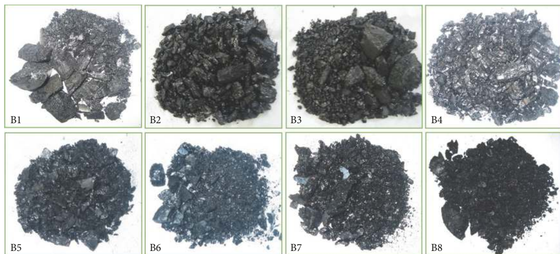
FIGURE 15: Failure forms of natural and 7D saturated specimens under uniaxial static-dynamic loads.
