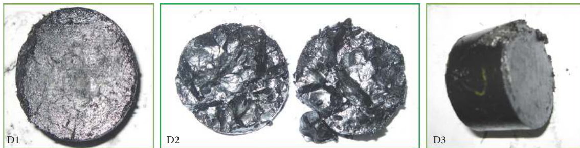
FIGURE 17: Failure forms of natural and water-saturated specimens under triaxial static-dynamic loads.
