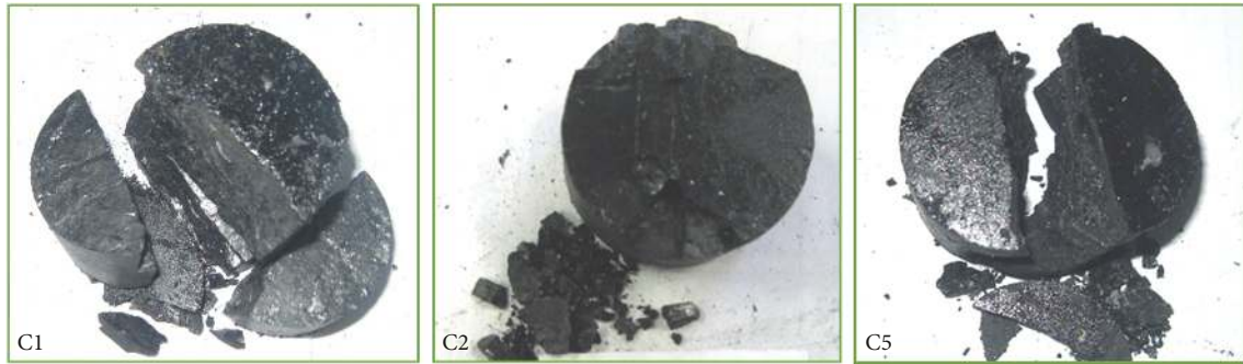
FIGURE 16: Failure forms of natural and water-saturated specimens under triaxial static loads.
