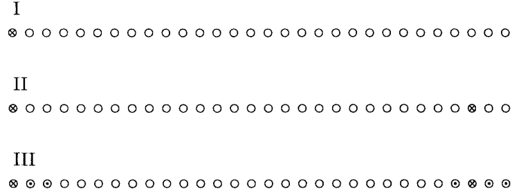
Figure 2. Snapshots of the failure process in a median strength ( N = 50 ) 1D HLLS \delta -bundle with 30 Weibull fibers for \rho = 10 and periodic boundary conditions. \circ intact fibers, \otimes broken fibers and \odot first failures after instability.
