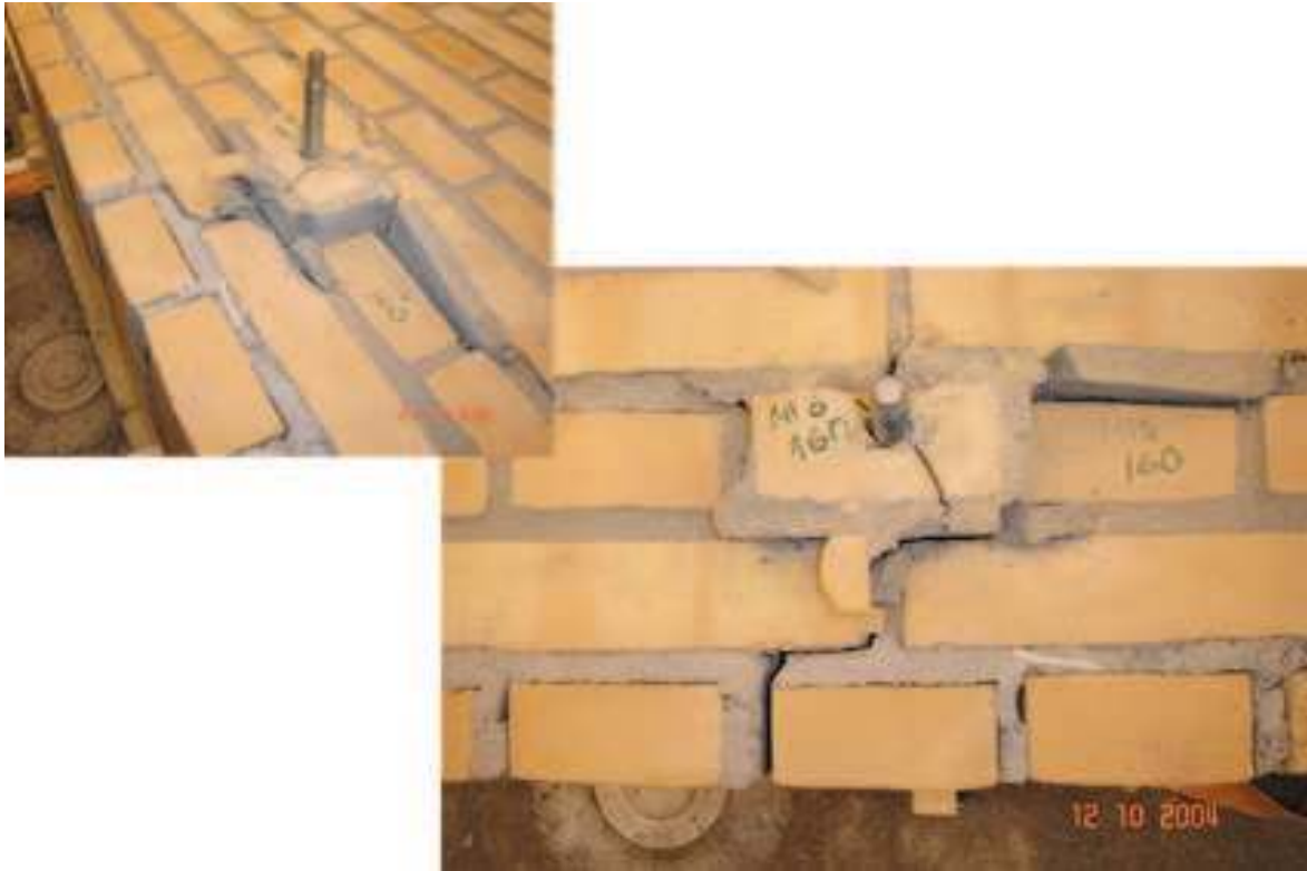
Figure A.147: The failure mode observed
