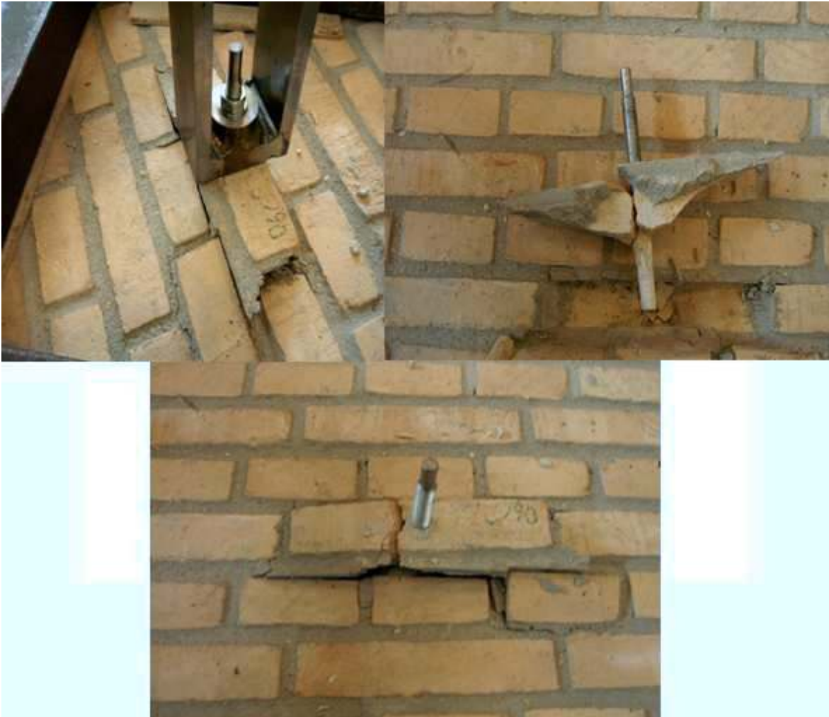
Figure A.35: The failure mode observed
