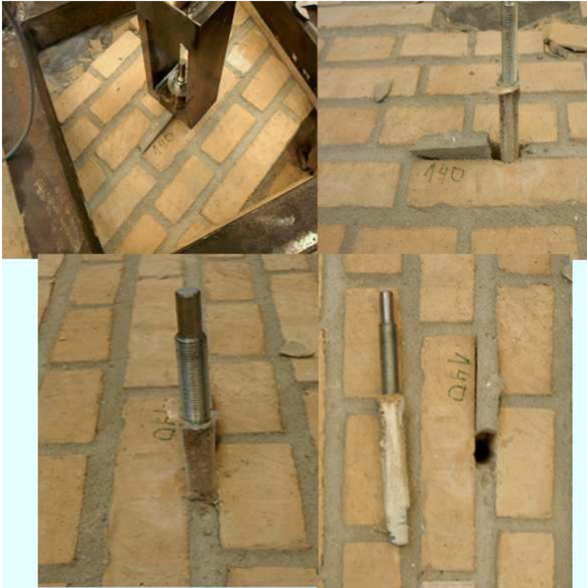
Figure A.105: The failure mode observed
