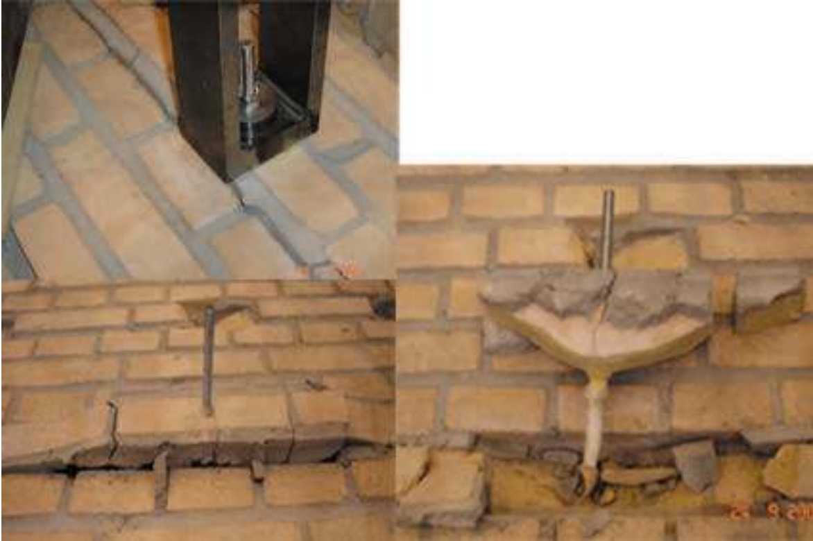
Figure A.5: The failure mode observed
