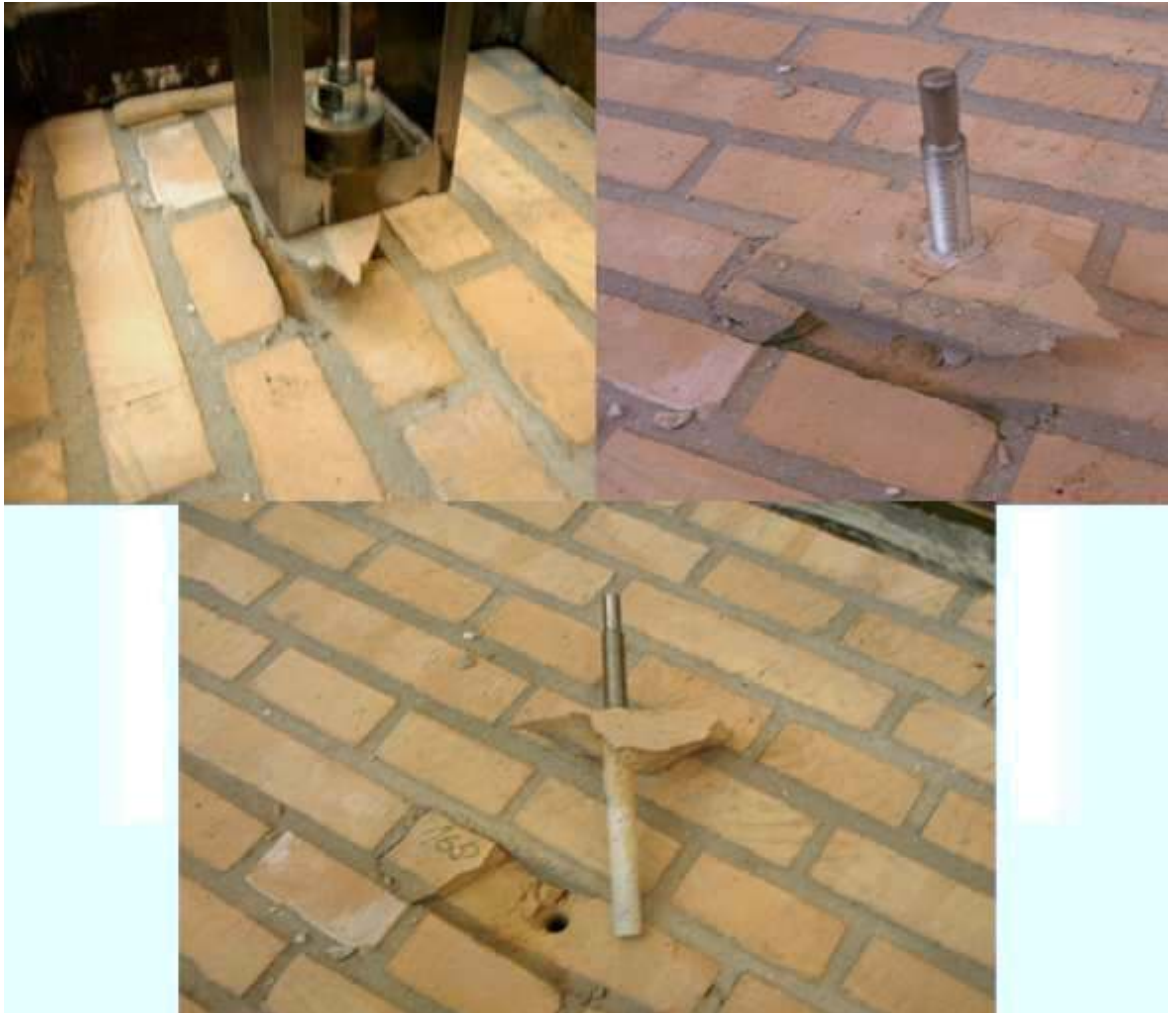
Figure A.37: The failure mode observed
