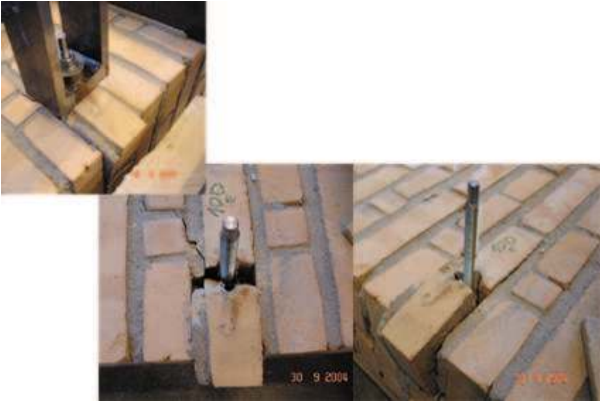
Figure A.133: The failure mode observed
