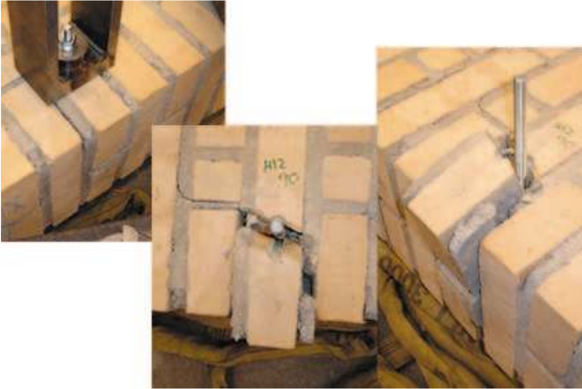
Figure A.127: The failure mode observed
