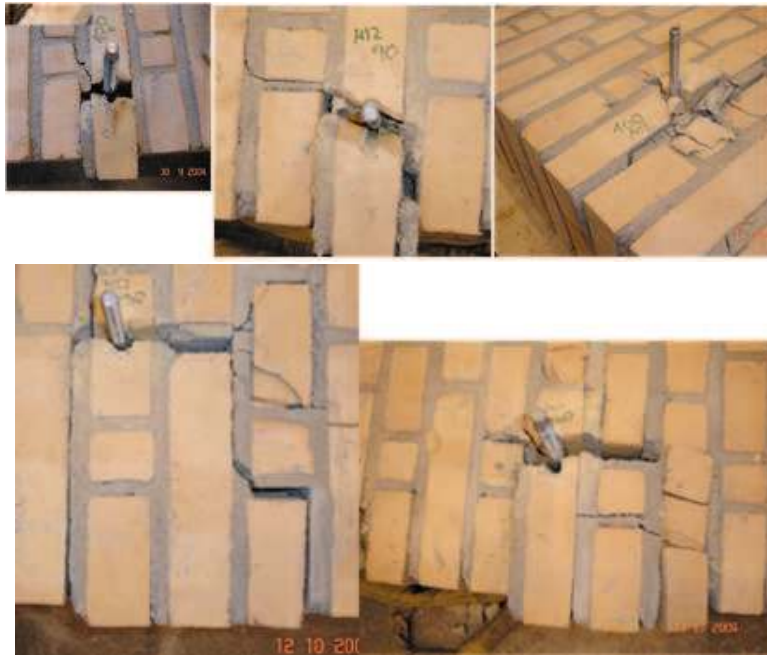
Figure 2.11: Typical splitting failures in masonry
