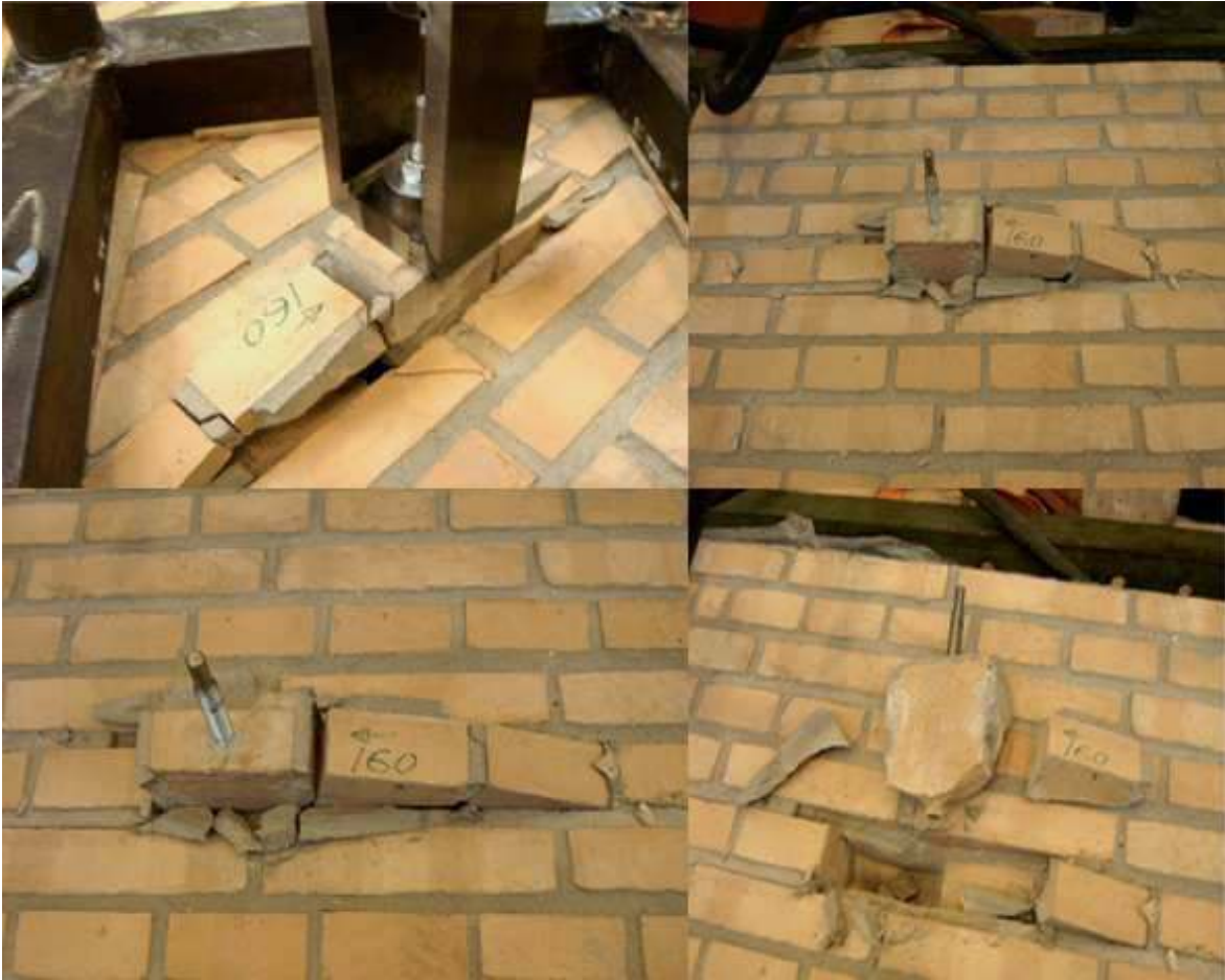
Figure A.83: The failure mode observed
