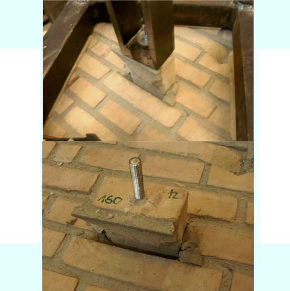
Figure A.75: The failure mode observed
