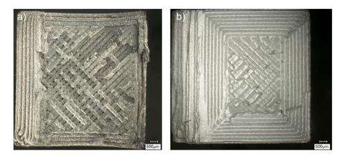
**Figure 16.** Fractured faces of the Charpy test metal FFF specimens presented as: (**a**) fractured surface (SEM image) of Ultrafuse BASF 316L specimen; (**b**) fractured surface (SEM image) of Markforged 17-4 PH specimen.
