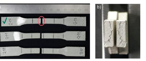
**Figure 8.** Fractures of tensile test BASF Ultrafuse 316L specimens presented as: (**a**) fractured specimens; (**b**) optical microscope image of the fracture surfaces, specimen 217. The samples have been numbered, which are visible in the figure. The letters L and R stand for the left-hand and right-hand sides of the sample in the figure. A green check mark means the specimen whose fracture faces were shown.
