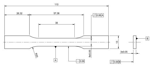
Figure 2. Tensile specimen design according to the standard [19], units: mm.
