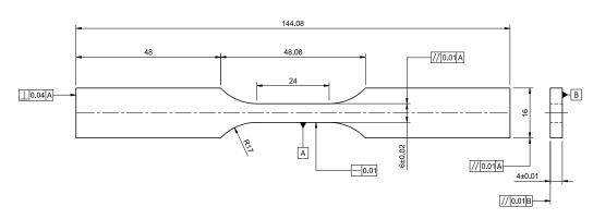
Figure 3. Fatigue specimen design according to the standard [20], units: mm.
