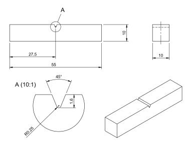
Figure 4. Charpy specimen design with the V notch according to the standard [22], units: mm.
