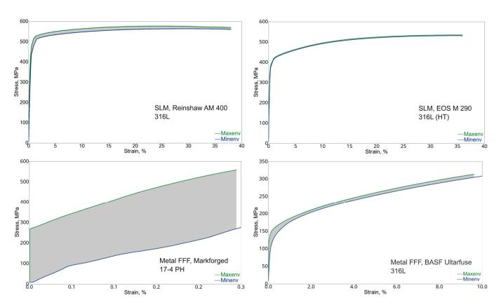
**Figure 6.** Envelope stress–strain curves (engineering stress versus engineering strain). Plots were created based on performed tensile tests considering all specimens.
