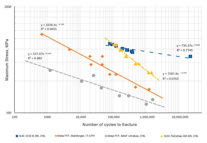
**Figure 11.** S-N curves for tested specimens; cycling tensile test with R = 0.1. (Two specimens of Ultrafuse 316L were broken in the grips, and their results were excluded.).
