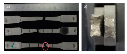
**Figure 9.** Fractures of tensile test EOS M 290 316L (HT) specimens presented as: (**a**) fractured specimens; (**b**) optical microscope image of the fracture surfaces, specimen 230. The samples have been numbered, which are visible in the figure. The letters L and R stand for the left-hand and right-hand sides of the sample in the figure. A green check mark means the specimen whose fracture faces were shown.
