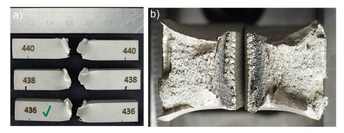
**Figure 17.** Fractures of Charpy test EOS M 290 specimens presented as: (**a**) fractured Charpy EOS M 290 specimens; (**b**) fracture surface (optical microscope image) of the EOS M 290 316L, specimen 436. The samples have been numbered, which are visible in the figure. The letters L and R stand for the left-hand and right-hand sides of the sample in the figure. A green check mark means the specimen whose fracture faces were shown.
