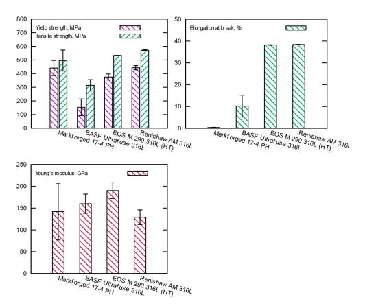
**Figure 5.** Results of tensile tests (mean with +/- standard deviation).
