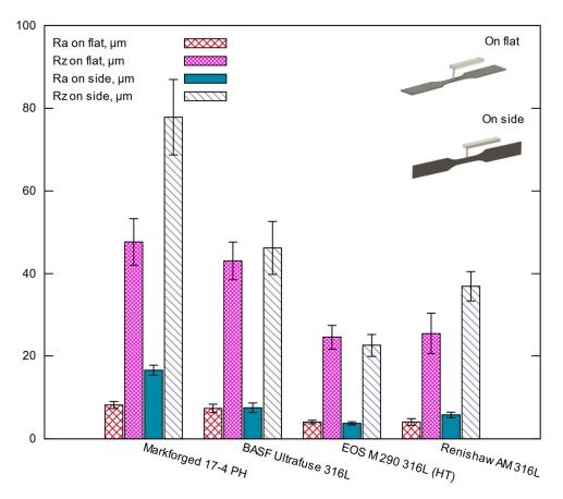
Figure 10. Results of roughness tests (mean  $\pm$  standard deviation).
