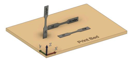
Figure 1. Printed specimen and predefined build orientations.
