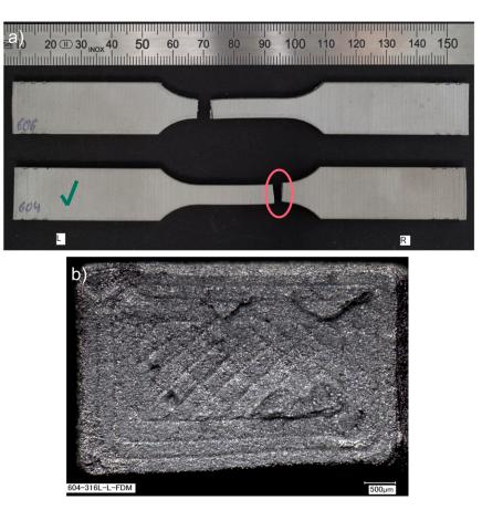
**Figure 13.** Fatigue fractures of BASF Ultrafuse 316L samples presented as: (**a**) fractured specimens during the fatigue test; (**b**) fracture surface (SEM image), left side, specimen 604, at 44,058 cycles. The samples have been numbered, which are visible in the figure. The letters L and R stand for the left-hand and right-hand sides of the sample in the figure. A green check mark means the specimen whose fracture faces were shown.
