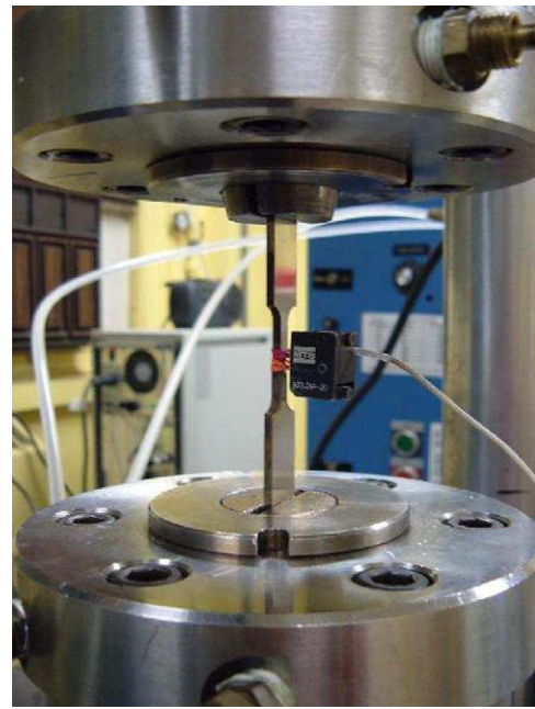
Fig. 2. Miniature extensometer attached to the test specimen.
