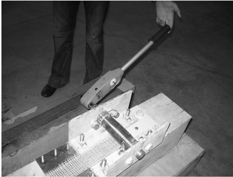
Figure 9. Prestressing technique: the metal cylinder.
