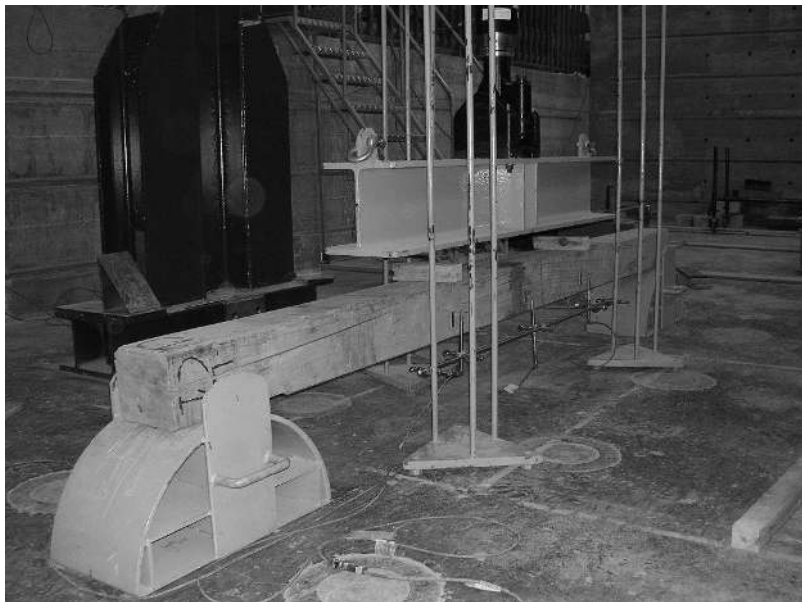
Figure 8. Flexural test set-up.
