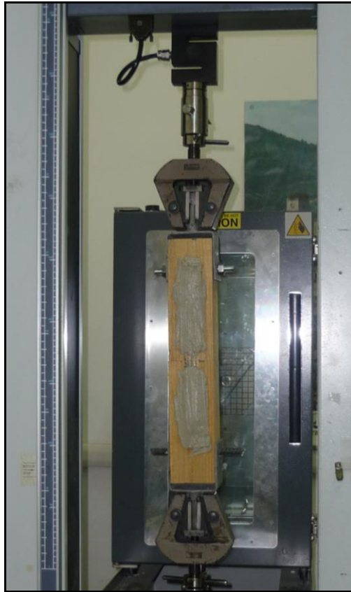
Figure 4. Layout of bond tests.
