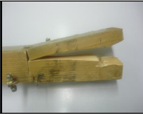
(b) Wood rupture.
