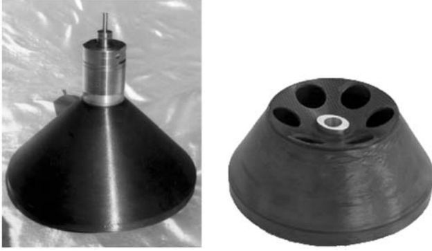
Fig. 1 Conical composite rotor ( \varnothing_a = 435 mm) and a composite centrifuge rotor ( \varnothing_a = 200 mm) [2]
