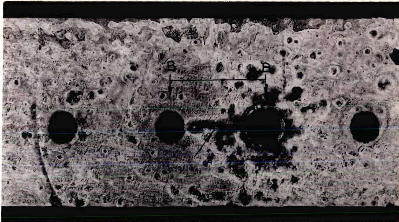
Detail A (Ref. Figure 12). Shown is the largest crack that appeared during the alternate immersion corrosion test. The crack extended between two of the stress coined holes and was aligned with the specimen longitudinal grain direction. Corrosion pitting is visible on the specimen surface. Section B-B is shown in Figure 14.
