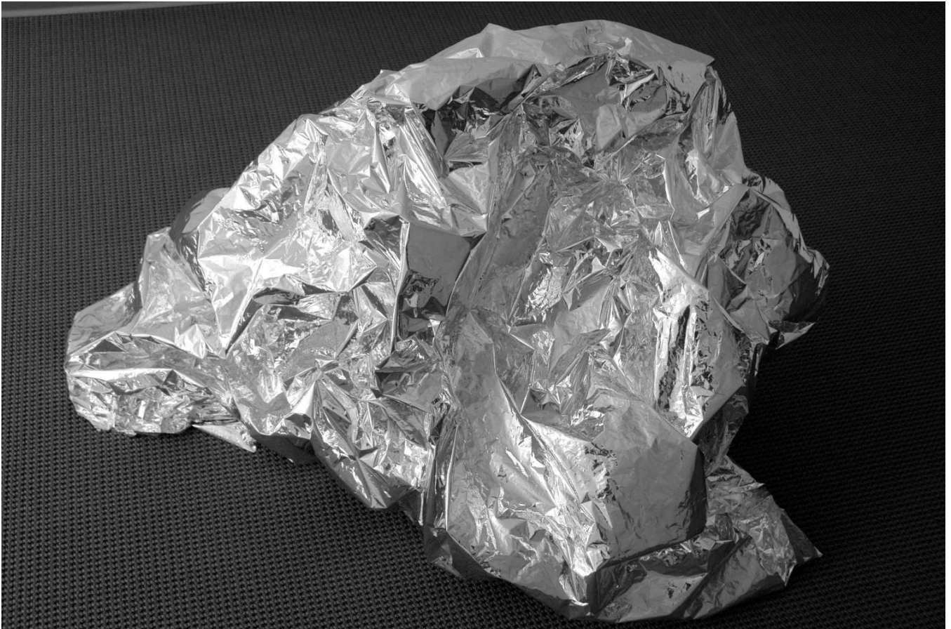
FIG. 1 A loosely crumpled sheet of aluminized mylar, 2 meters in width and 10 microns in thickness, courtesy of Henry Frisch
