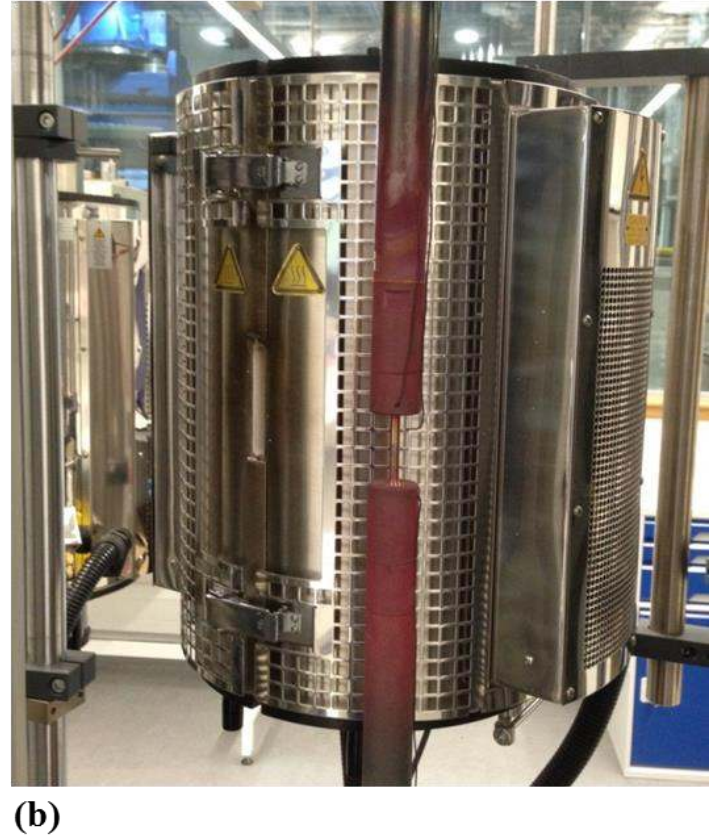
Figure 3: (a) The mechanical model used to represent the elastic and plastic deformation in stress relaxation tests; \sigma_e , \sigma_i , and \sigma_0 are effective stress, internal stress and applied stress, respectively, (b) a photograph showing the tensile test rig taken just after the termination of a test at 720°C.
