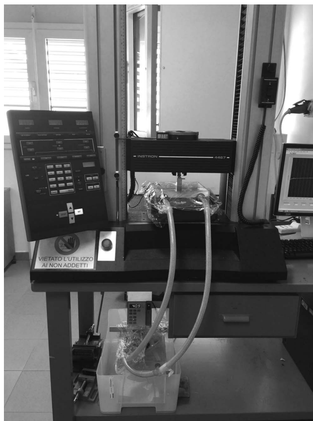
Figure 2. Hydraulic circuit to keep the temperature constant.
