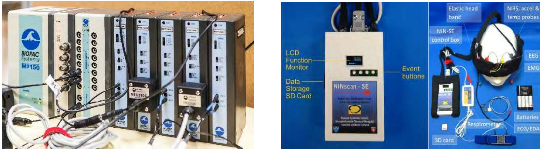
FIGURE 11. Laboratory version of IOMS-SRA system based on BIOPAC MP150 vs. field-deployable NINscan system for ambulatory brain and physiologic monitoring in operational environments.
