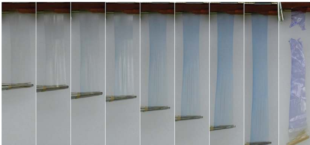
FIGURE 4. Photo series displaying mechanochromism in PCL film 6 as it is deformed to failure.
