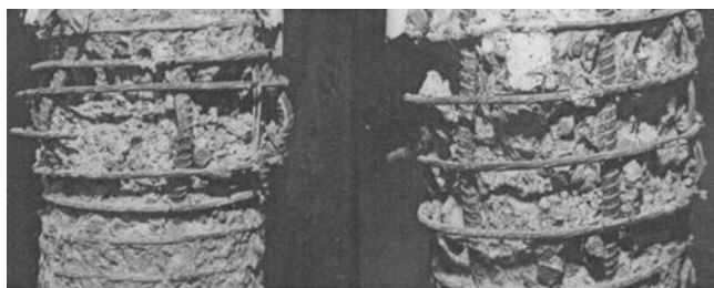
Fig. 9—Specimens with ultra-high-strength ( f_{yh} = 1318 \text{ MPa} ) confining reinforcement after testing.
