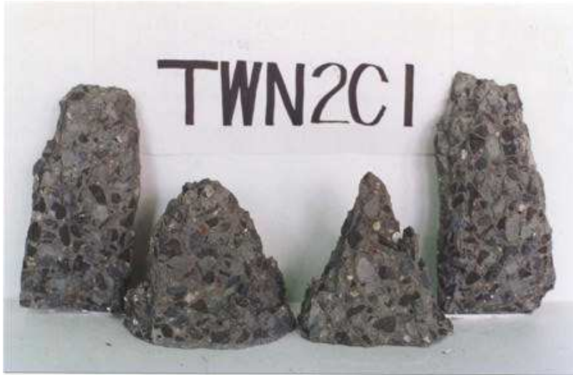
Fig. 12 Failure Mode of typical HSC specimen (without steel fiber) at 100°C
