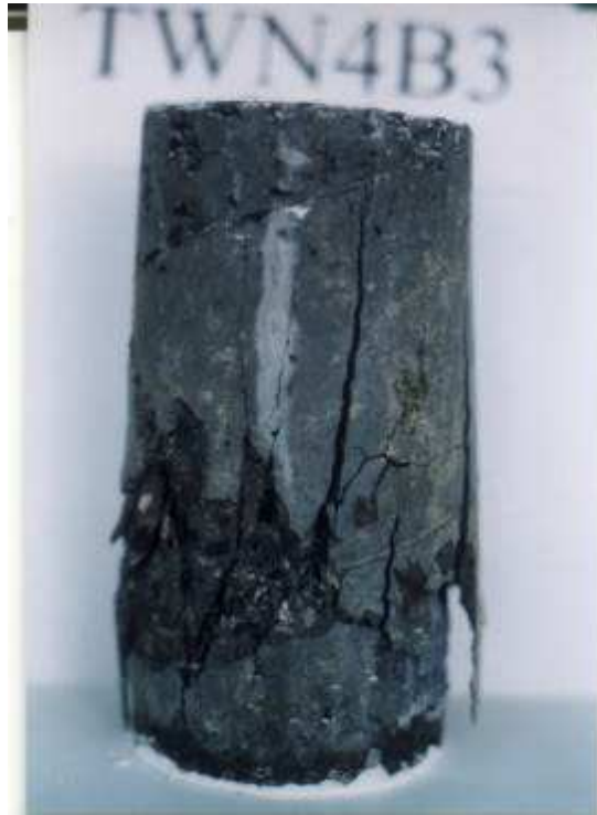
Fig. 14 Failure Mode of typical specimen (with steel fiber) at 100°C
