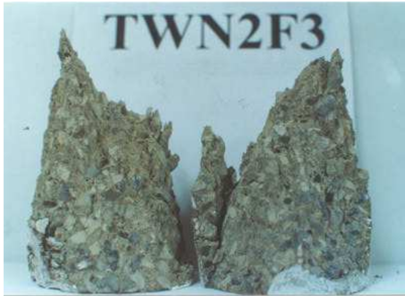
Fig. 13 Failure Mode of typical HSC specimen (without steel fiber) at 800°C
