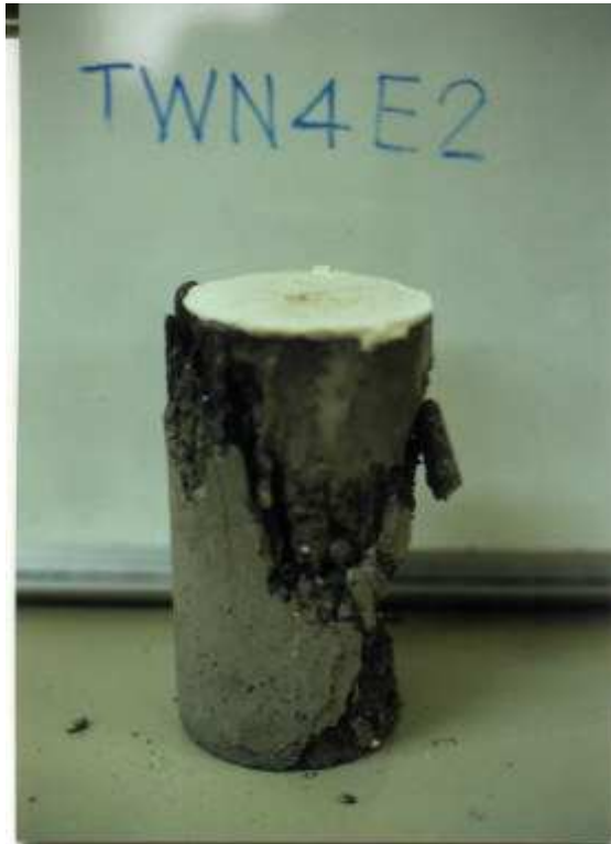
Fig. 15 Failure Mode of typical specimen (with steel fiber) at 800°C
