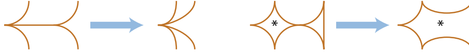
Fig. 12. The simplification operations that transform an outerplanar strict confluent drawing into its canonical diagram: contraction of arcs without sharp angles at both ends (left) and merger of marked faces and triangles (right).
