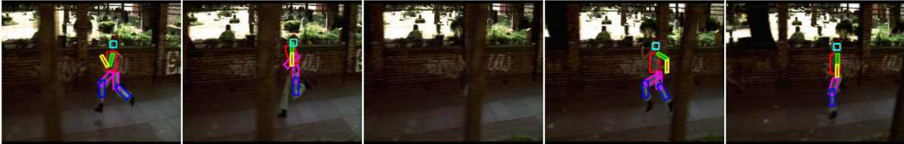
Figure 11. Automatic tracking of one of the shots from the 30000 frame 'Lola' sequence. Even though the figure is performing a fast running motion, the arms and legs are quite well localized. The track recovers from the full occlusion of the telephone pole and handles self-occlusion as well.
