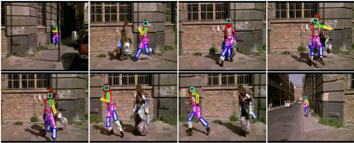
Figure 4. A sequence from ‘Lola’ of Lola running around corner and bumping into a character while undergoing extreme scale changes. Note the character is wearing bulky clothing and so our person detector has no hope of finding him. Our initial walking detector is run at a single scale; once we learn an appearance model (as shown in Fig.2), we track over multiple scales by searching an image pyramid at each frame.
