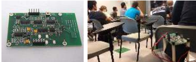
Fig. 1. The BumbleBee sensor is a monostatic wideband radar, with a bandwidth of 100MHz, a center frequency of 5.8GHz and a maximum detection range for people at \sim 10 m omnidirectional.
