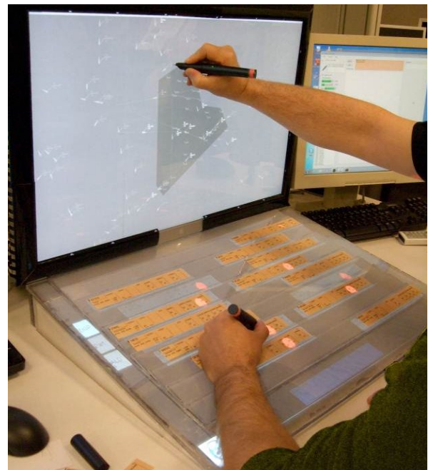
Figure 1: two controllers using the Strip'TIC prototype (digital pens, augmented radar, stripboard, and paper strips).
