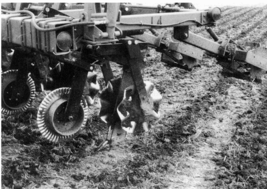
Fig. 2. A shank/coulter strip tillage machine used in the 1999 and 2000 experiments.
