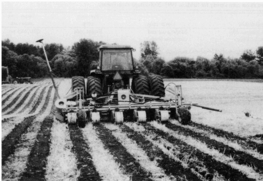
Fig. 1. A rotary strip tillage machine used in the 1997 and 1998 experiments configured to till six rows 20 cm wide on 75-cm centers.
