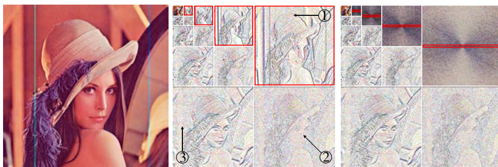
Fig. 3. Original Lena image impaired by two vertical stripe offsets (left). The wavelet decomposition up to the level 4 is visualized in the centre. The low pass coefficients c_l are displayed at the upper left, the horizontal details coefficients c_h for each decomposition level are displayed in the vertical row to the left (3), the diagonal detail coefficients c_d in the diagonal row (2). The striping noise is condensed to the vertical details coefficients c_v in the horizontal row at the top (1). The details bands that are affected by the vertical striping noise are enframed with red boxes (only as qualitative markers). After applying the 2D Fourier transforms to those bands (right), the information of the striping noise will be completely condensed to the abscissa. The transforms have been applied to each R, G, B channel separately and overlaid to color wavelet coefficients.
