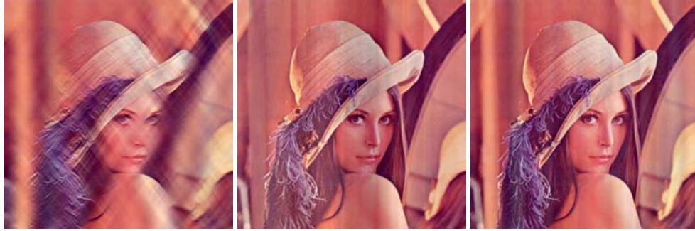
Fig. 4. Stripes elimination from the original Lena image (Fig.3, left) by using different strategies. The left image displays the result after removing the relevant vertical details bands [1] (wavelet: DB42), the centre image shows the result of damping the horizontal frequencies in \hat{x} for \hat{y} close to zero, and the right image displays the results of the combined method proposed in this work.
