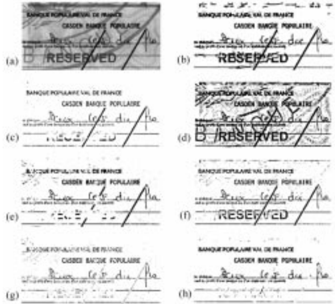
Fig. 9. Local binarization results of "French Cheque." (a) Raw image; (b) enhanced Bernsen's method; (c) Kamel-Zhao's logic level technique; (d) Oh's LLT based on bright-average scheme; (e) Tophat Transform followed by Ostu's method; (f) Niblack's method; (g) Djeziri's filiformity followed by Ostu's method; and (h) proposed double-edge followed by conditional dilation.
