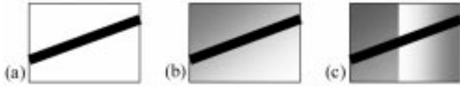
Fig. 1. Character stroke on different types of background. (a) Simple background; easy to binarize by global thresholding; (b) slowly varying background; can be removed by local thresholding; (c) fast varying background; need to be removed by feature thresholding.
