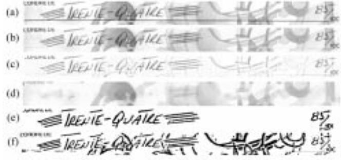
Fig. 6. An example of Legal Amount extraction. (a) Raw image A (1341 \times 99 pixels); (b) new image A' after baseline removal; (c) double-edge feature detected in image A'; (d) background image estimate from image A'; (e) character extraction by feature thresholding; and (f) binarized image by applying Bernsen's algorithm to the raw image A'.
