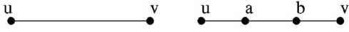
Fig. 2. Each edge e = (u, v) in G = (V, E) is replaced by three edges (u, a), (a, b), (b, v) in G' = (V', E') .
