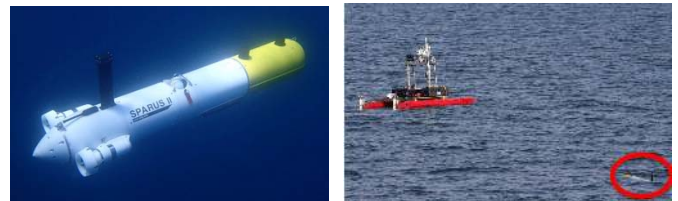
Fig. 1- a) SPARUS II AUV. b) ROAZ II ASV and SPARUS II AUV at surface.
