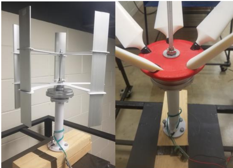
Figure 3.12. ALEKO WGV15 Assembly (left). Test hub design installed on ALEKO hub (right).
