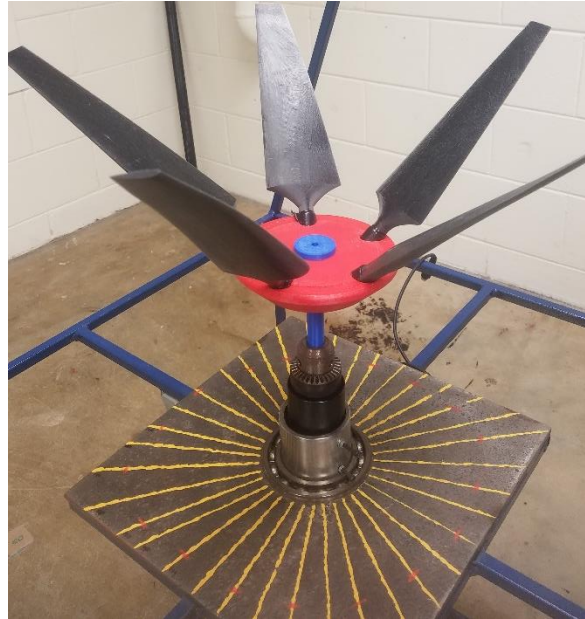
Figure 3.17. Torque test assembly, with shaft lock-up.
